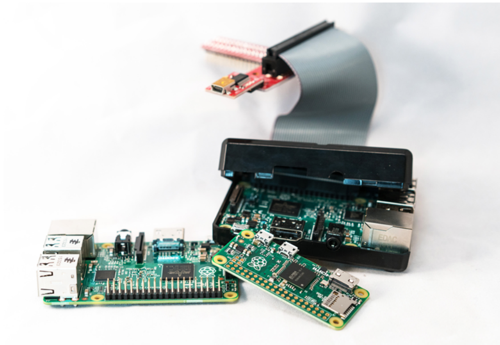
Figure 11.2 Raspberry Pi 2 Model B (left), Raspberry Pi Zero (center foreground), and Raspberry Pi 3 Model B (in a case, with attached SparkFun Pi Wedge)
